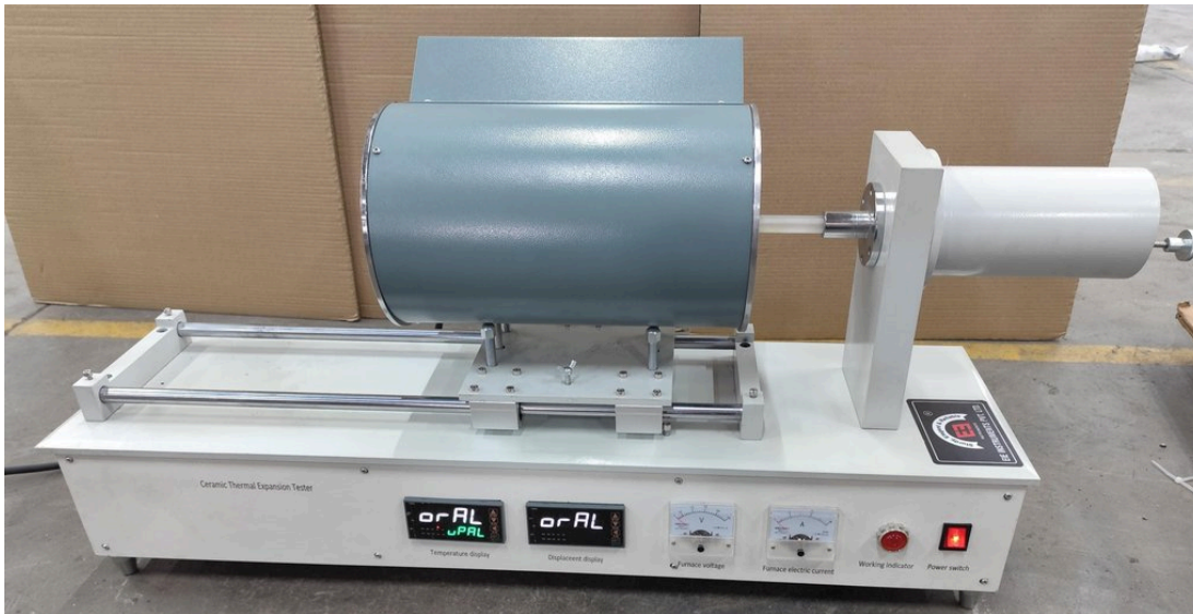
DILATOMETER-DETERMINATION OF LINEAR THERMAL EXPANSION-1400 °C
